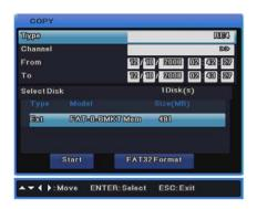
You can back up videos using HDD or USB storage. You can play them using the mini player or network manager. Select the channel field and use the [Enter] button or the mouse wheel to open the channel list as shown below.
